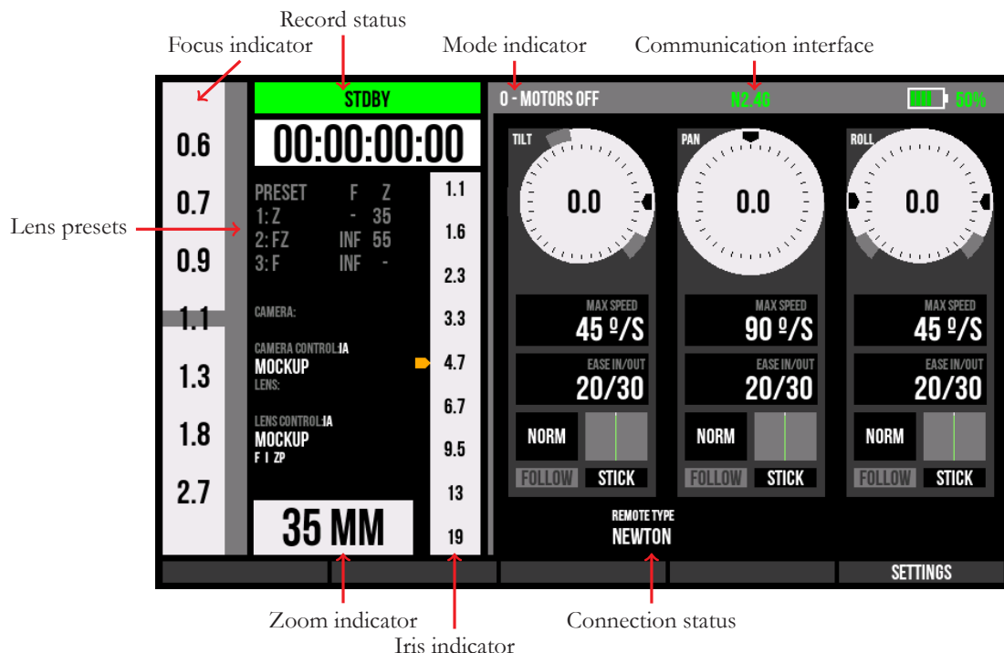
Figure 4.1: Newton Controller Main Page
